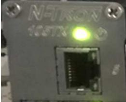
Connect one end of an Ethernet cable to the computer which will transfer files. The other end of the cable should be inserted into a free jack on the Ethernet switch which the PLC is connected to.
